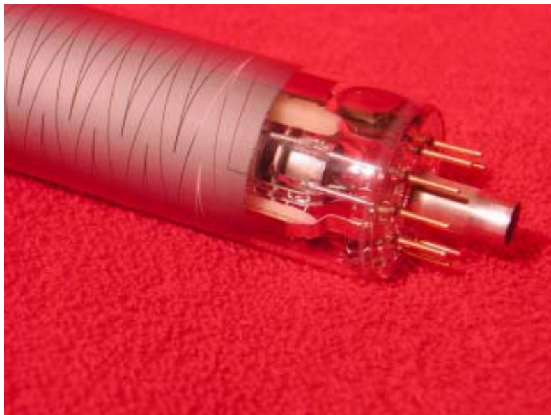
Figure 7 Zigzag Deflection plates (From the author's collection)
