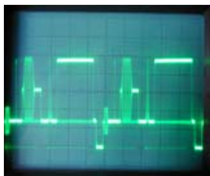
Received pulse and bar test signal on a scope (line rate)
